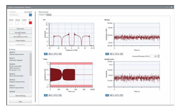
Characteristic parameters may be streamed continuously to Host-PC to get reports over long-term tests. Complete received spectrum may be stored in intervals of typical one second for informational or debugging purposes. Data is reduced effectively by down-sampling mechanisms.
