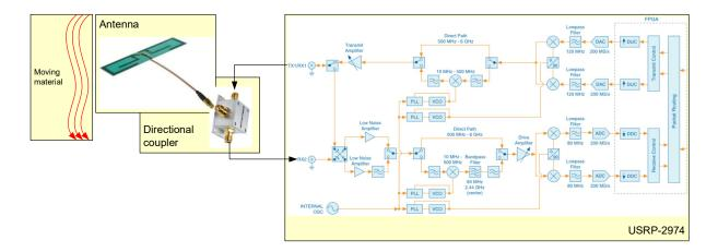
An electrical antenna is positioned close to the material under test. The SDR-device transmitter sends a stimulation signal to the antenna via the directional coupler. Depending on the frequency, the RF energy is partially reflected, back to the SDR-device. The directional coupler makes sure that the reflected energy is fed back only to the SDR-device receiver.
