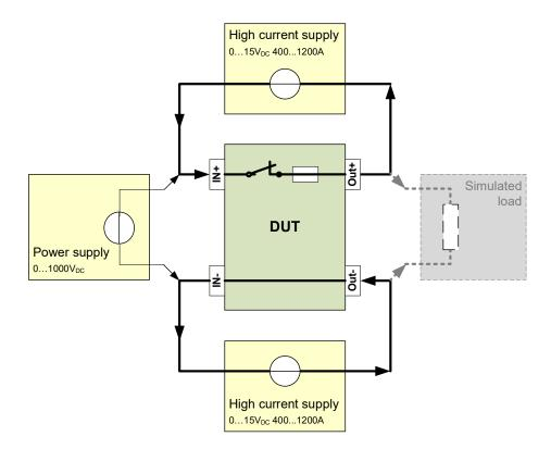
Please note, that not every low voltage power supply is capable of handling such high battery voltages. Choosing the right device is crucial for proper operation of such a setup. The same principle may be applied at various applications, where both high voltages and high currents are necessary. IRS has not only built such systems for battery junction boxes, but also for testing of automotive power connectors.
