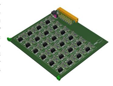
IRS provides a modular cell simulation for 24 cells on a single board. The cells on the simulator can be combined in series and several simulator boards are cascadable for higher voltages.
