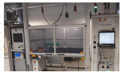
Battery junction boxes for electrical vehicles may include isolation monitors. Since only one isolation monitor may be active at the same instant, flexible isolation monitors are used in the test system, which can be deactivated at certain test steps.
